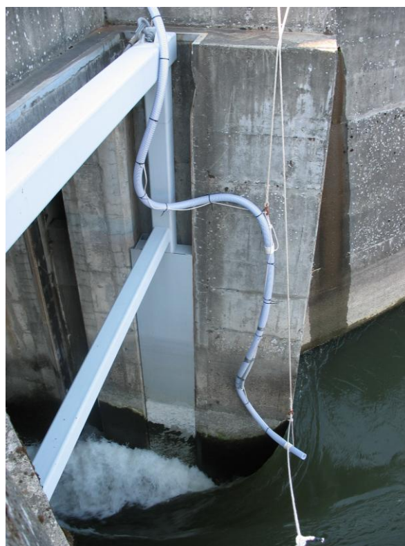
Figure 6. Photos of the setup used to suspend the 4-inch hose in front of the entrance to the corner collector. By adjusting the guide lines attached to this hose, we could position the hose to different locations for releasing fish in front of the entrance. These photos show the middle and north release locations.
