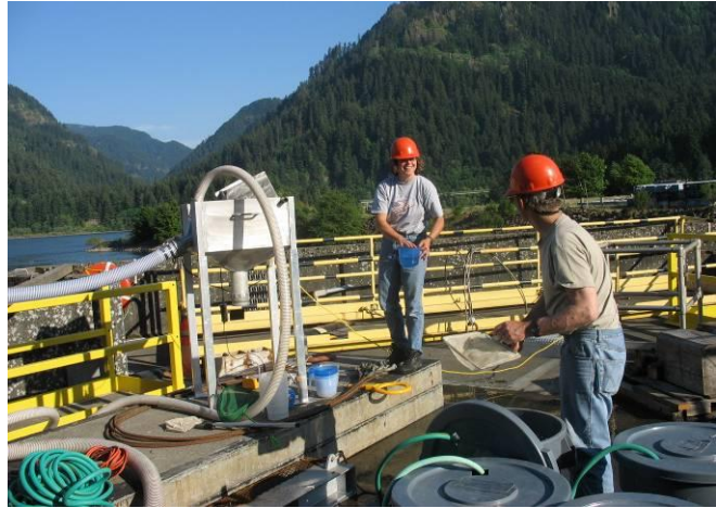
Figure 13. Powerhouse deck above the entrance to the corner collector where fish were released. Flush water was added to the 4-inch hose to keep fish moving through the hose.
