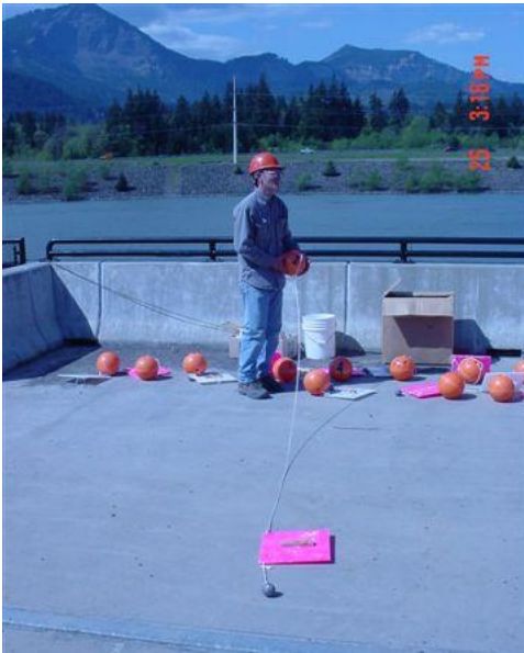
Figure 2. Photo of floating drones designed and released by NMFS. The tags were inserted into wooden blocks fastened onto plastic vanes, which were connected to floats with three lengths of rope (the one shown yielded a tag passing through the antenna near the bottom of the flume). A 12-oz ball weight was attached at the bottom to help maintain orientation.
