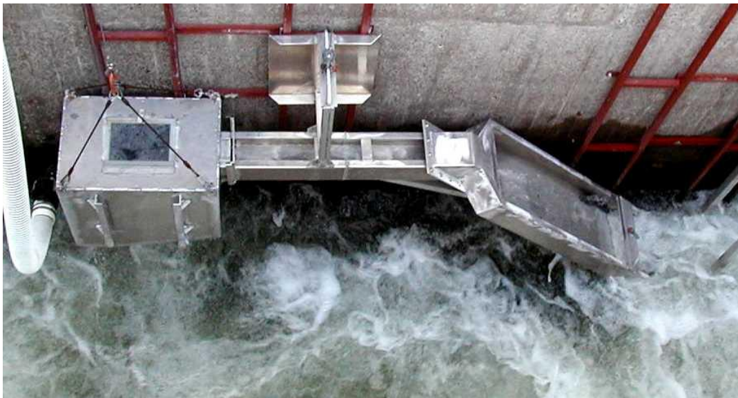
Figure 4. Bypass collectors tested in 2002 and 2003 at the Bradford Island MWC. The top photo shows the closed tube design and the bottom photo the open ramp design. Both collectors featured a trap box at the upstream end (left side of photos) that could be lifted independently to enumerate lamprey.
