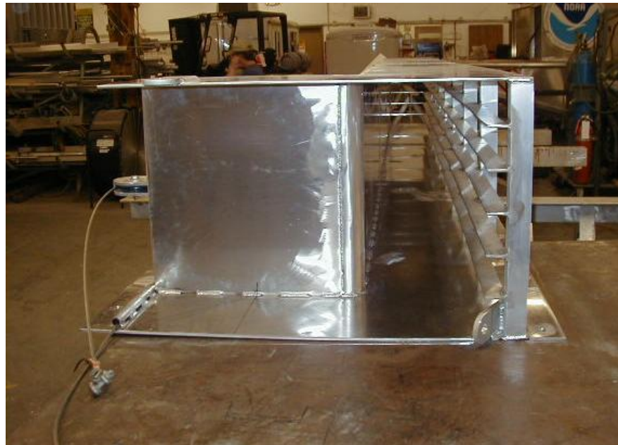
Figure 11. Transition structure (top view) to guide lamprey into the collector and provide a seat for the collector base. The structure was fabricated at the Northwest Fisheries Science Center Pasco Research Station. Bars were attached to prevent sea lions from accessing lamprey as they climb up this submerged structure.
