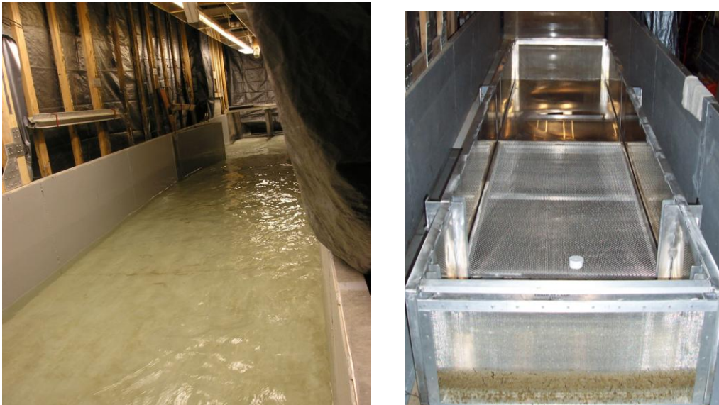
Figure 3. Experimental covered flume area at the McNary juvenile bypass channel (left) and flume insert apparatus shown in the dewatered flume (right).
