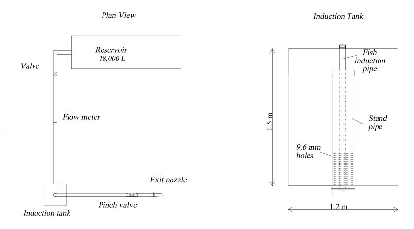
Figure 1. Plan view of test area and close-up view of fish induction tank used for the high-velocity induction/release tests at NMFS Pasco Field Station, fall 1998.
