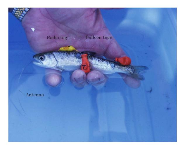
Figure 2. A tagged juvenile chinook salmon used in tests at NMFS Pasco Field Station during fall 1998. The balloon tags are the "Hi-Z Turb'n Tags" (non-inflated), and the lighter colored tag is a radio-tag (with antenna).
