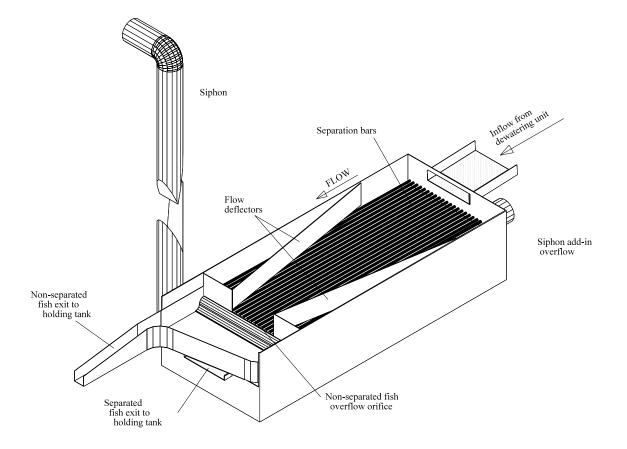
Figure 1. Components of the simulated conventional wet separator used for wet-separator efficiency development studies at McNary Dam in 1999.
