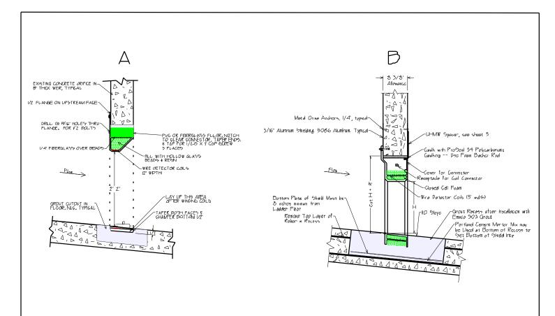
Figure 1. Cross-section drawings of the original 5-inch chamfer antenna-housing design (A) used in the AFF during 2000 and the final 1-inch chamfer antenna-housing design (B) that will be produced for the 2001 installations. Note the increased coil width and the increased separation between the coil windings and the water in B.
