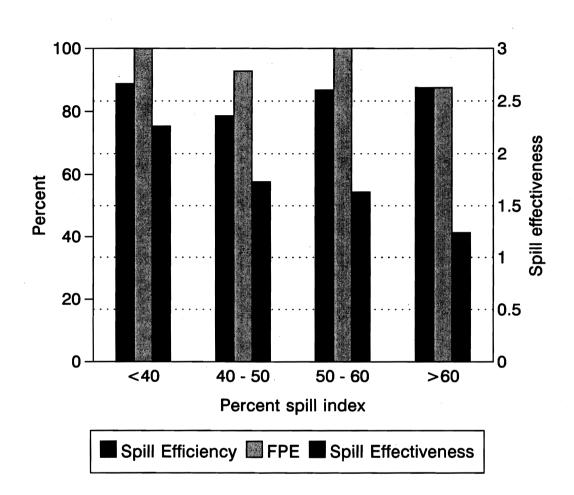
Figure 8. Spill efficiency, spill effectiveness, and fish passage efficiency (FPE) for radiotagged hatchery-reared subyearling chinook salmon at Ice Harbor Dam, 1997.
