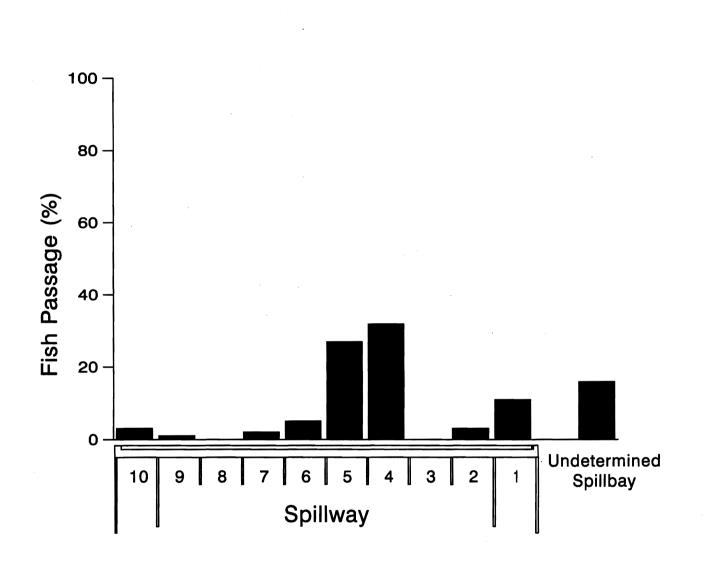
Figure 6. Spillway passage distribution for radio-tagged hatchery-reared subyearling chinook salmon at Ice Harbor Dam, 1997 (Spillbays 3 and 8 were closed throughout the duration of the study).
