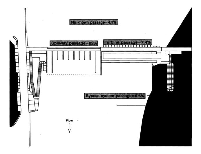
Figure 5. Passage distribution for radio-tagged hatchery-reared subyearling chinook salmon at Ice Harbor Dam, 1997. (Note: Radio-tagged fish with records on the entry and exit lines but with no record of passage at the dam were assigned turbine passage).
