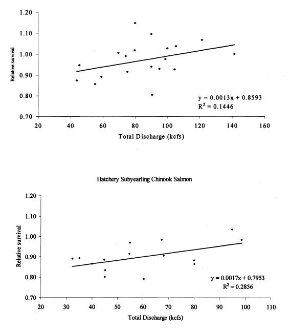
Appendix Figure D4. Estimated relative spillway passage survival by total dam discharge at time of release for PIT-tagged hatchery yearling and subyearling chinook salmon released at Ice Harbor Dam, 2000.
