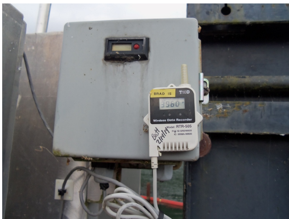
Figure B9. Wireless data recorder, RTR-500.
