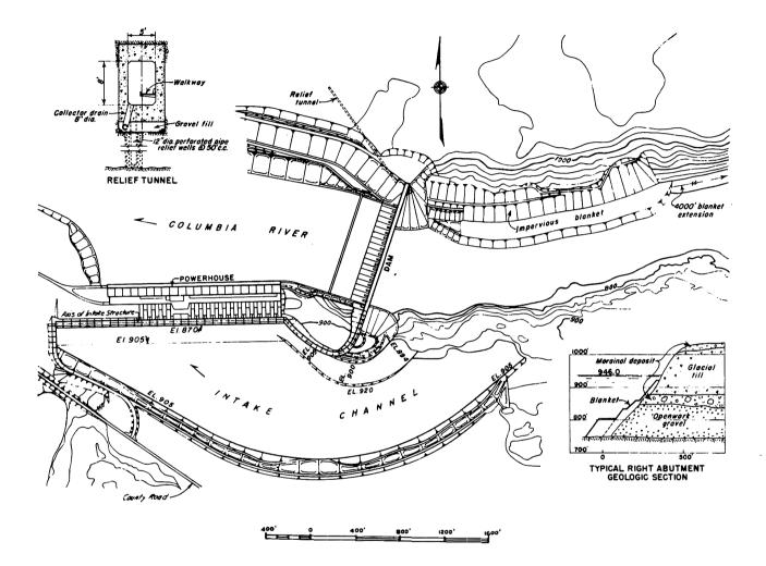
Figure 1.--General layout of Chief Joseph Dam with details of impervious blanket and relief tunnel required to control seepage in the right abutment.
